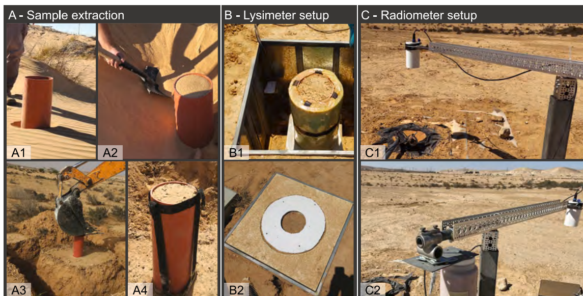
Fig. 2. Lysimeter preparation (A) and set-up (B) and radiometer deployment (C). The sand sample was filled by hand (A1–2), while the loess sample was an undisturbed soil column (A3–4). After sealing the samples at the bottom, they were insulated with spray foam, and placed on a balance inside a pre-installed metal container, flush with the soil surface (B1). A Styrofoam block with a cylindrical opening for the lysimeter was mounted on ledges inside the metal container (B2). After covering the Styrofoam block with a thin layer of soil, the radiometer was attached to a moving arm next to the lysimeter, and set to move between the lysimeter (C1) and the reference standard (C2).
